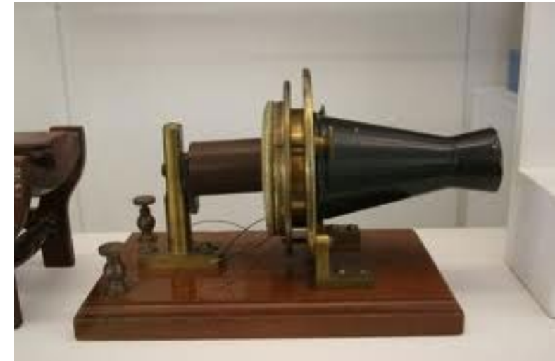
Alexander Graham Bell telephone prototype, 1876
